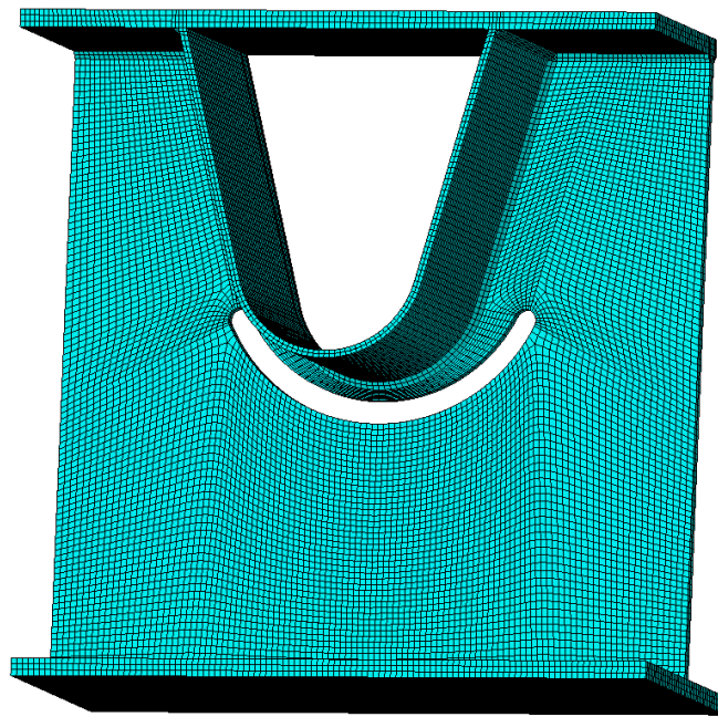
Figure 25. Illustration. Submodel C mesh at RFB connection. Average mesh size is \frac{1}{4} inch.
